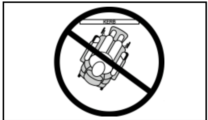
Figure 3. Incorrect Kerb Approach
