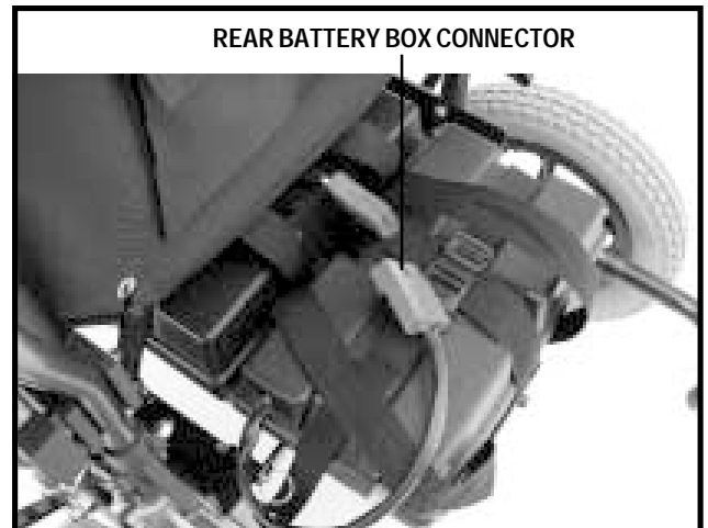
Figure 7. Rear Battery Box
