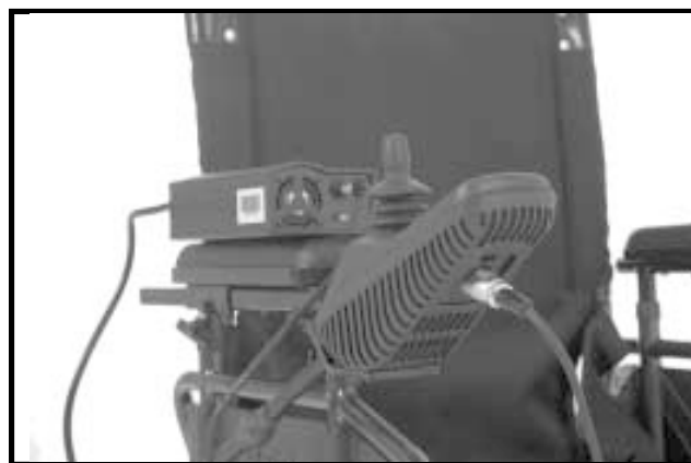
Figure 22. Charging the Batteries
