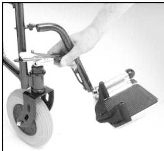
Figure 20. Foot Rigging Installation
