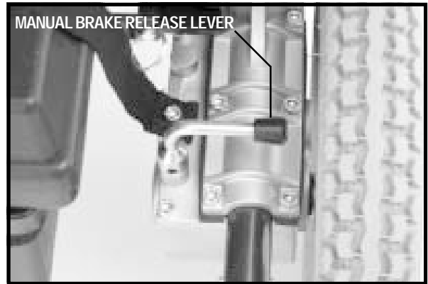
Figure 9. Drive Motors Disengaged (Freewheel Mode)
